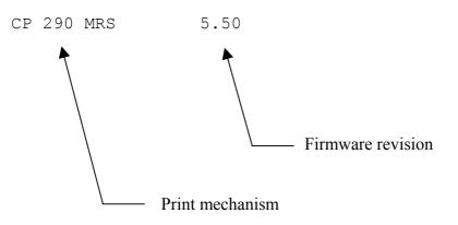
Note : The string always has a fixed format, that is : the print mechanism name padded to 16 bytes, a space, then 5 bytes for the firmware revision (the dot being in the middle), ended with zero.
