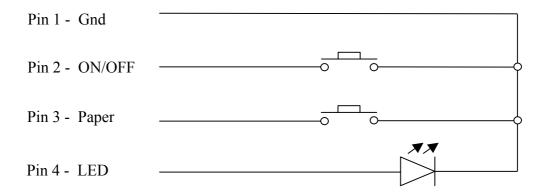
(\*) A serial resistor (470 Ohms) is on the printer, setting the LED current at about 7 mA.
