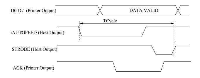
In this mode, the data transfer controlled is given by the host, but tCycle must not exceed 0.5 seconds
